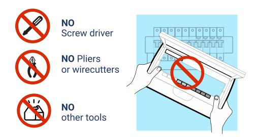
**DO NOT** remove cover or any shielding to access electrical wires or cables.
